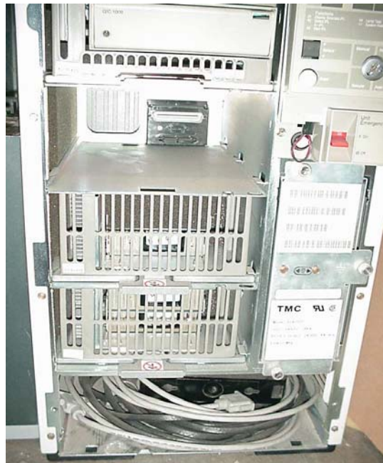
IBM AS/400 System with Drive Bays Exposed
